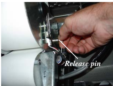
Figure 6-8. Release pin location.
