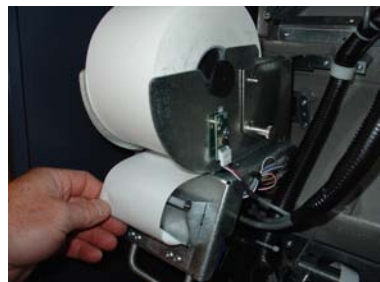
Figure 6-6. Feed paper into slot.
