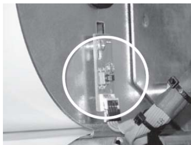
Figure 6-2. Paper feed button is located on the paper bracket.
