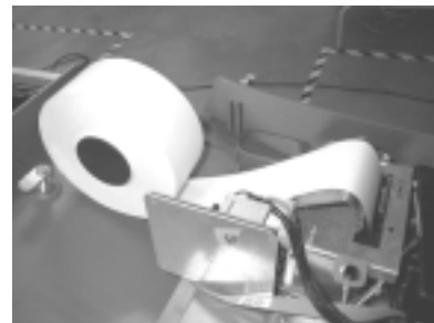
Figure 6-7. A new roll of paper installed on the Printer.
