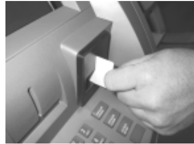
Figure 6-8. Use the cleaning cards on a monthly basis to maintain effective card reader operation.
