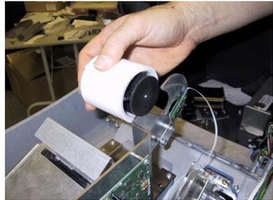
*Figure 6-3. Removing paper roll from bracket.*
