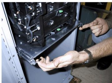
Figure 4-1. Lift up on slide tray locking levers.
