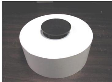
*Figure 6-4. Insert spindle into new paper roll.*
