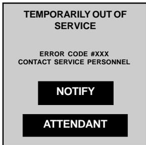
*Fig. 7-1. The 'Out of Service' screen is displayed if the terminal detects an error condition.*
