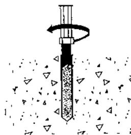
Figure 6. Drive anchor rod into capsule using hammer drill.
