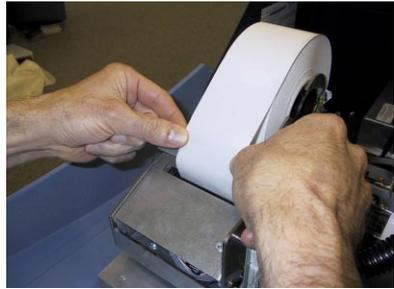
*Figure 6-6. Feeding paper into the printer take-up slot.*
