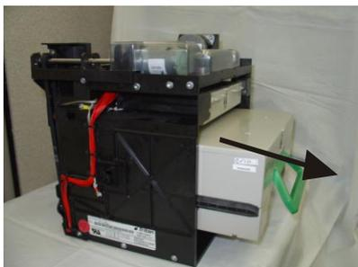
*Figure 4-6a. Removing note cassette. (TDM-100)*
