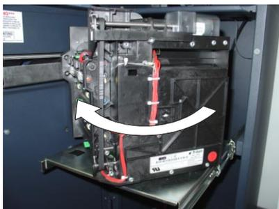
*Figure 4-4. Rotate mechanism to service position (clockwise).*
