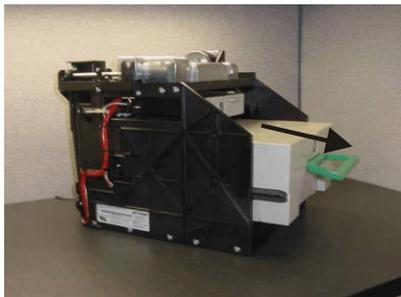
*Figure 4-6b. Removing note cassette. (TDM-150)*
