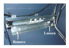
Pivot each slide rail slightly inward. This will allow easier access to secure the nuts to the plinths mounting screws when installing the ATM cabinet..
