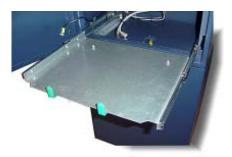
Locate the locking slide tabs on each side of the slide rails. Push tabs up/down on each side and remove tray from rails. Push rails back into cabinet and set tray aside.
