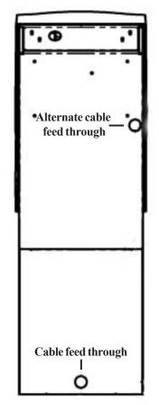
Figure 2. Power and phone cords routed through either access hole.
