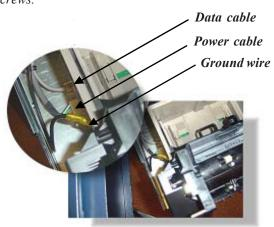
Figure 6. Dispenser cable connections.
