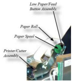
Figure 6-1. Printer assembly.
