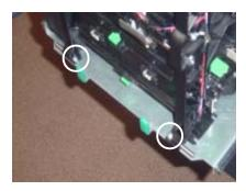
Figure 5. Install front mounting screws.
