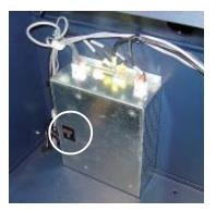
Figure 1. Power switch location.
