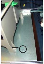
Figure 4. Align slots of dispenser under screws.
