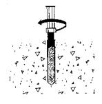
Drive anchor rod into capsule using hammer drill.
