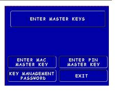
Enter Keys - Enter the first (32) alpha/numerical key. The on-screen keypad legend describes the ATMs keypad for entering numbers and characters. Select "ENTER" using the display function key.
