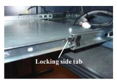
Using a phillips screwdriver, remove the two (2) front screws that secure the rail assemblies; retain screws. Next, *loosen* the back screws.
