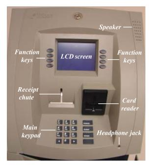
Figure 2-1. Control panel layout.
