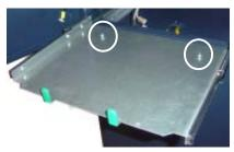
Figure 3. Loosen phillip screws in rear mounting holes.
