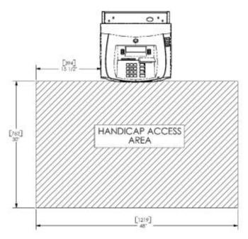
Figure 7. Handicap access area.
