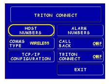
Note: Comms Type Option For Model 8100/9100 ATMs, this function detects the communication type installed (wireless) and <u>will not</u> allow user to change (toggle).
