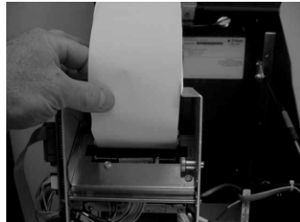
Figure 6-7. Paper feeds automatically when placed in take-up slot.
