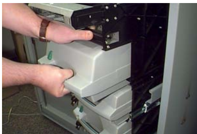
Figure 4-16a. Removing the reject vault.
