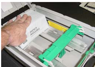
Figure 4-12. Leveling note pile.
