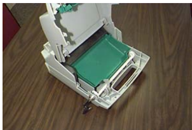
Figure 4-19. Bundle reject tray.
