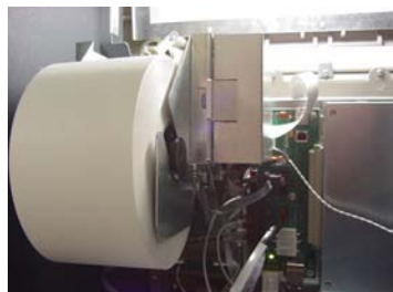
Figure 6-5. Paper on bracket.
