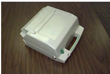
Figure 4-16b. Reject vault ready to open.
