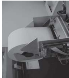
Figure 6-6. Paper feeds from top of roll.
